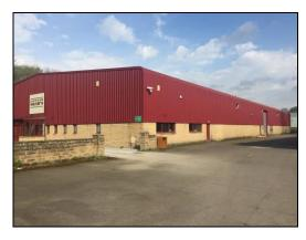
In addition, to the rear of the main building (Unit 1) there is a brick built single storey industrial/warehouse building (Unit 2) being part timber metal clad under a 'belfast roof' which is supported on large timber trusses with perspex roof lights and hasbeen re-clad. This building benefits from a concrete floor and some ancillary provisions.
